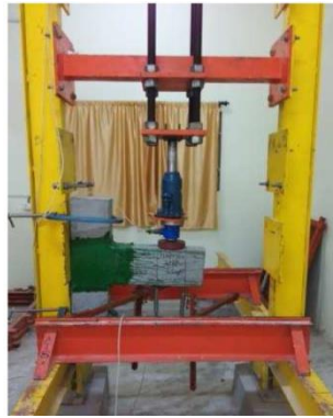
Figure 6. Testing of beam-column specimens in the loading frame
