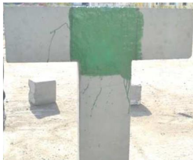
Figure 5. Application of the first layer of mix over the concrete.
